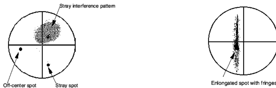
Figure 3: Stray interference patterns in microscope view. Figure 4: Stretched spot in microscope view.
